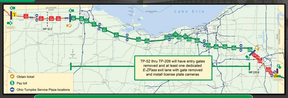
Convert Eastgate toll collection to one-way WB (into Ohio and opposite to Penn Turnpike Gateway which is tolled one-way EB)
