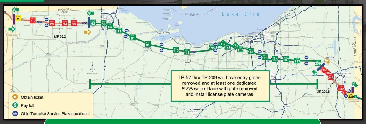
Construct two new mainline plazas with highway speed E-ZPass lanes at MP 49 and MP 211 (new ends of closed ticket system)
